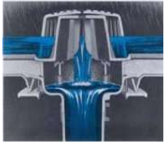
Zurn Run-off limiter – Typical
